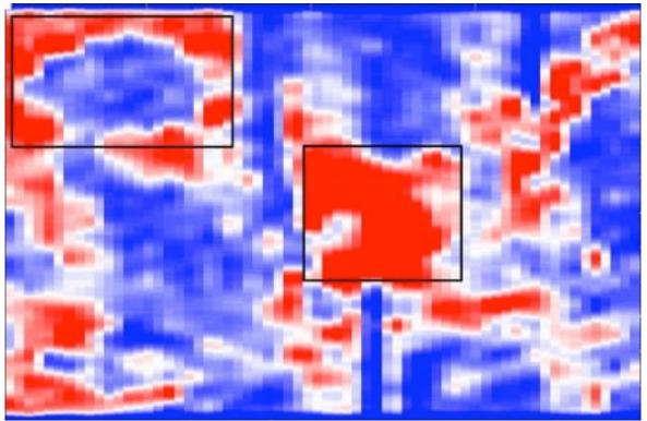
Fig. 14. Ground-penetrating radar profile (October 16-17, 2003) showing buried rectangular feature (upper left) and solid feature (center). 1/2 inch = approx. 6 ft.; Depth: 1.5 ft.
