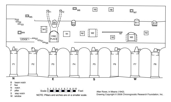
Fig. 3. Unfolded elevation of inside Tower wall (after Rowe, in Means, 1942).
